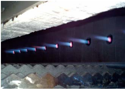
Fig. 3. WS REKUMAT burners firing in “flame” mode with 90% POC extraction. The walking-beam rails are shown in the foreground.
