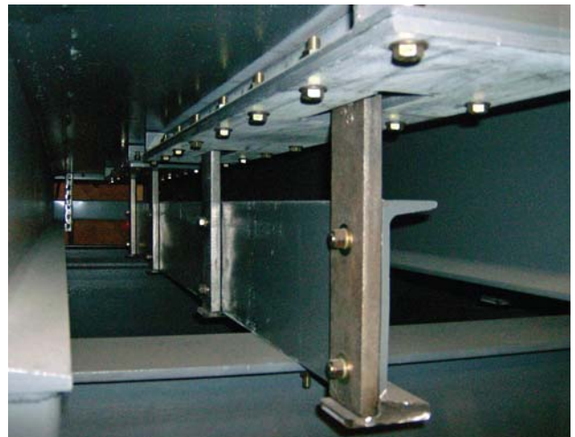
Fig. 2. TNI's hearth and walking-beam design provides very low heat loss through the hearth.
