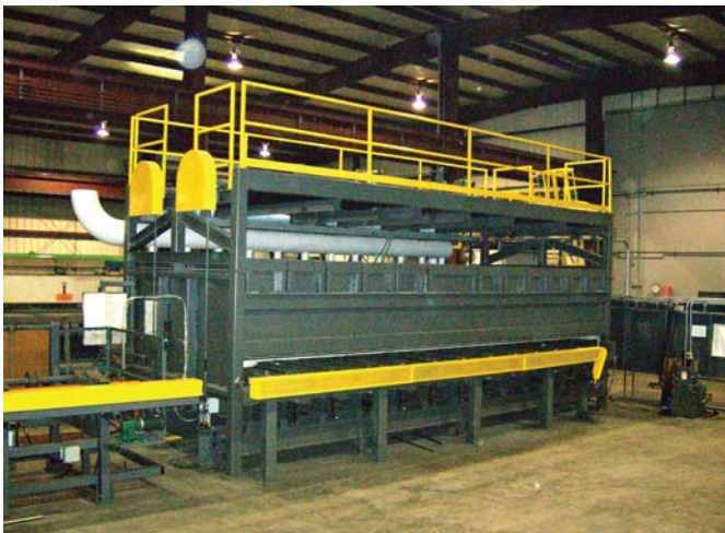
Fig. 1. The TNI walking-beam furnace showing the bar loading system.
