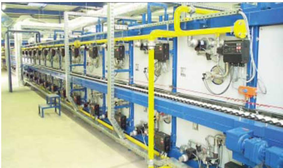
Selection of components depends on the choice of temperature control. In a frequency-fired system, select components that allow on/off cycling of each burner using direct-spark ignition.
