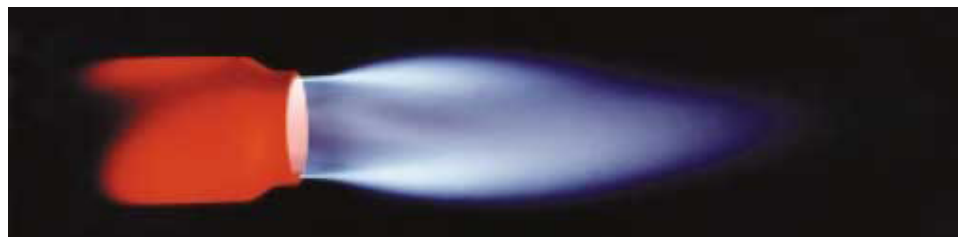
When selecting the right burner for your application, determine the burner capacity, ratio requirement, flame shape, turndown capability and outlet velocity. All of these aspects of burner operation play a key role in the successful operation of the system. (Shown is the Kromschroder modular design BIC burner.)
