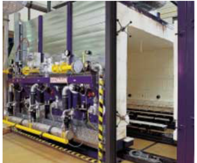
While burners are an essential part of any combustion system, the fuel train, combustion blower, flame safety system and temperature control system are equally important.
