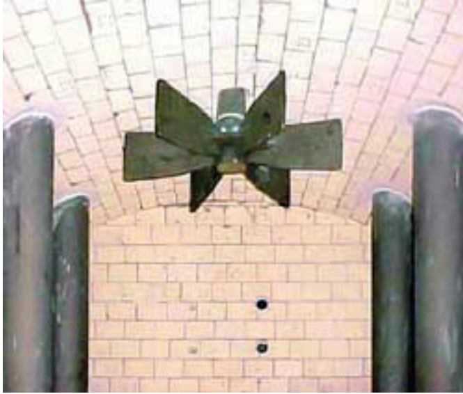
Vertically mounted APM radiant tubes have a projected service life of 4-6 years.
